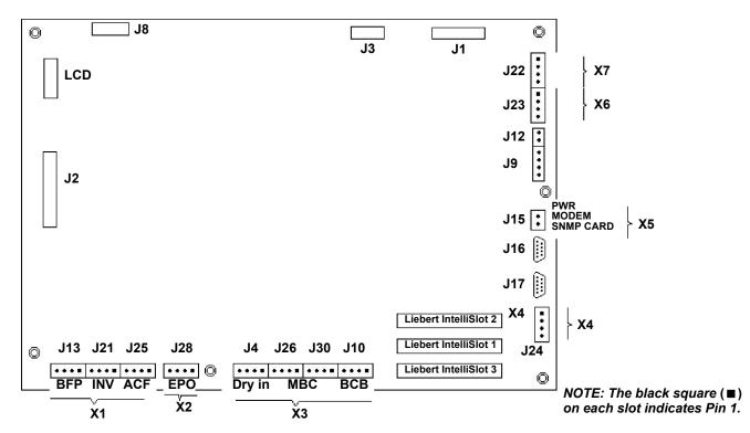
Figure 5 Auxiliary terminal block detail (Monitoring Board)
